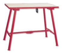
2 types of professional workbench for the heating specialist and plumber: - Multi-ply wooden worktop edged with steel angle section frame, Ø 40 mm tubular legs for model 200910, - Multi-ply wooden worktop, Ø 35 mm tubular legs for model 200920. Very sturdy construction, able to support heavy loads. Easy to set-up, take-down and carry. Wide base ensuring high stability. Foldable with locking device.
